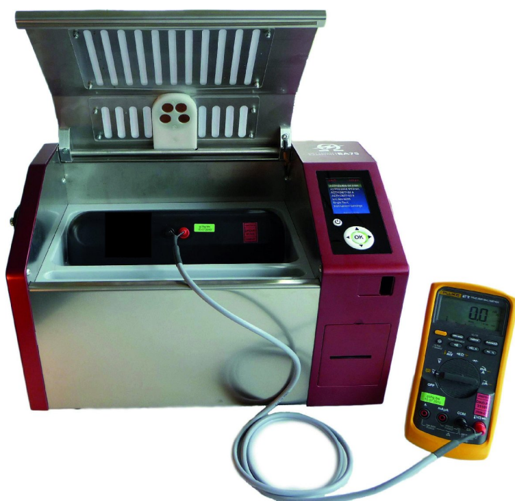
Picture: Test set-up VT75 with BA75 and Fluke multimeter
